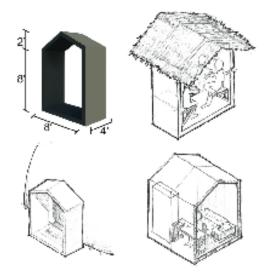
Figure 3. Basic design of proposed prefabricated component with possible configurations.
