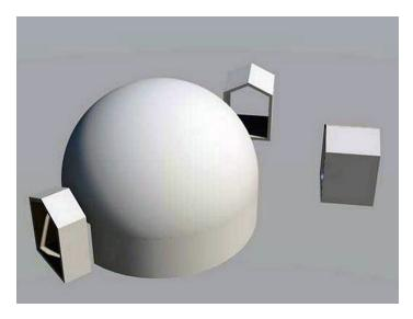
Figure 4. Possible layout of additional prefabricated components and their connection to dome house.
